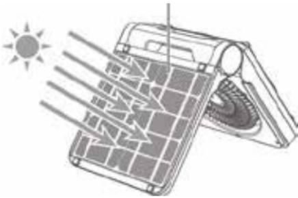
1. The integrated solar cell continuously converts ambient light into energy that is utilised for charging the appliance. However, since the suitability of light sources such as fluorescent lamps and other interior lamps is limited, we recommend that you charge the appliance by sunlight.
